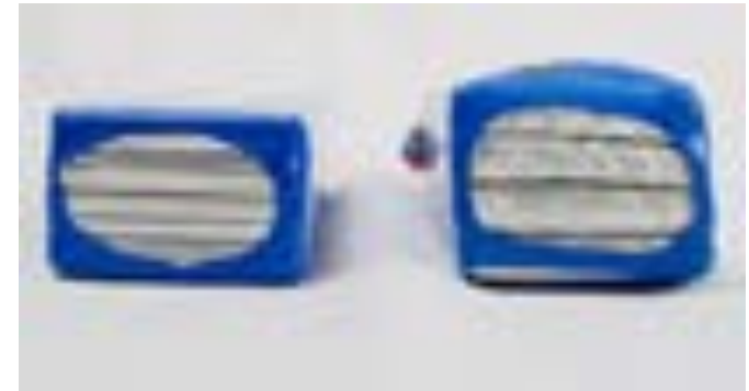
Battery swelling caused by overcharging
